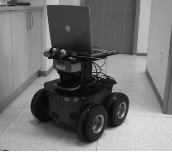
Figure 1. Wheeled Pioneer 3-AT mobile robot with laser range scanner Sick LMS200.
